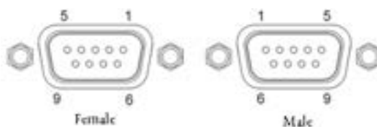
Figure 2.1.3.7.2 Pin descriptions of the CONTROL interface
