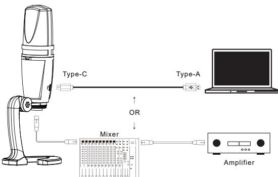
**Method 1:** Use the included USB cable to connect the JS-1P Plus at the Type-C end and the computer at the other end.
