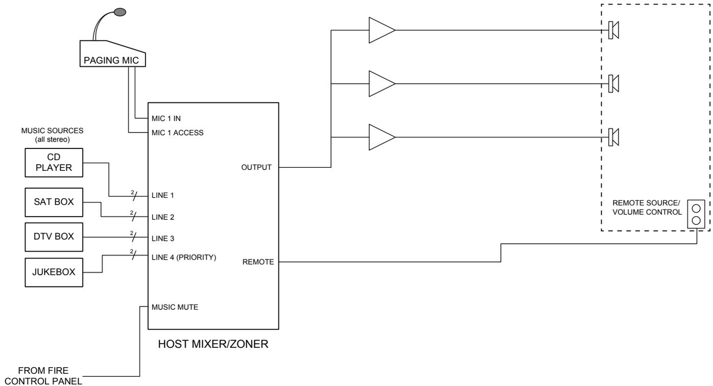
The diagram shows a PMI microphone connected to a “generic” mixer or zoner, together with a variety of music sources. Provided the host device is correctly configured, pressing the PMI’s PTT switch will automatically mute the selected music source and allow paging from the microphone.
